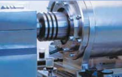
*Test rig for rotary shaft seals with PTFE sealing lip for testing various parameters.*
