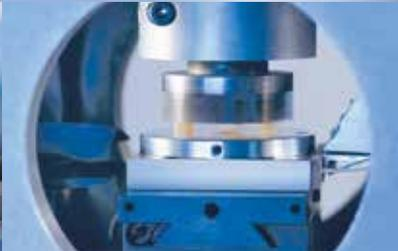
*Test rig for long-term wear rates of PTFE compounds with various sliding mates.*
