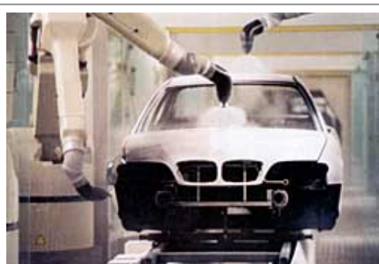
Painting process in the automotive industry Picture: Dürr Systems
