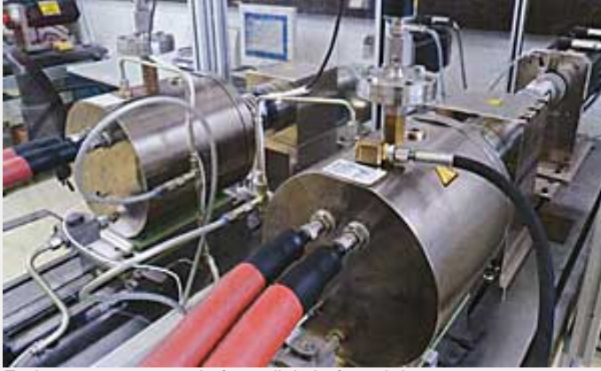
Endurance wear test rig for radial shaft seal rings.
