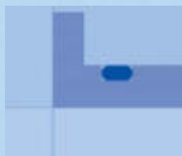
Clamping flange with additional O-ring seal.
